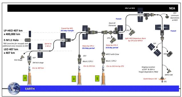
Figure 11 – Design Reference Mission for Crewed NEA Mission using Advanced Propulsion
